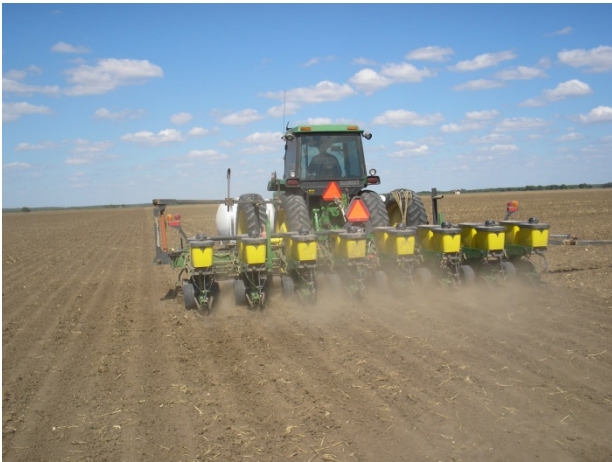
Photos 17-18. Nearly all planters can be adjusted to plant sesame in many row spacings, conventional to no-till, beds or flat.
